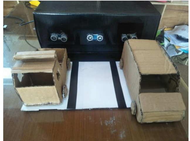
Fig. 6 Ultrasonic Sensor Testing at a Distance of 3 cm
