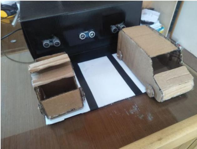
Fig. 4 Implementation of a Car Parking Distance Controller
