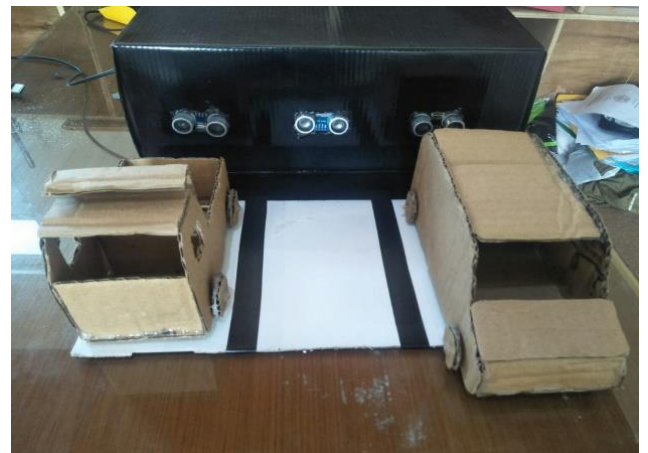
Fig. 7 Ultrasonic Sensor Testing at a Distance of 2 cm
